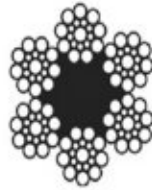
6x19 constructions. Suitable for general engineering purposes, winch, pulling and marine applications. (HR-4 rope)
