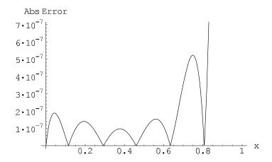
Fig 6 Absolute error between exact and approximate solutions of Eq. (3.18)
