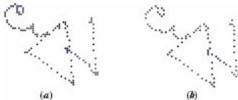
Figure 4. (a) Sampling points of an input character with 3 strokes, (b) The same character after first resampling.
