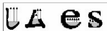
Fig.14. Identification procedure of some of the English and Japanese characters considering upper part of top reservoir.
