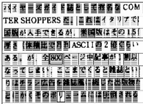
Fig.16. Identification results of our proposed system. (portions marked by horizontal line segments are identified as Japanese text, and rest are English).
