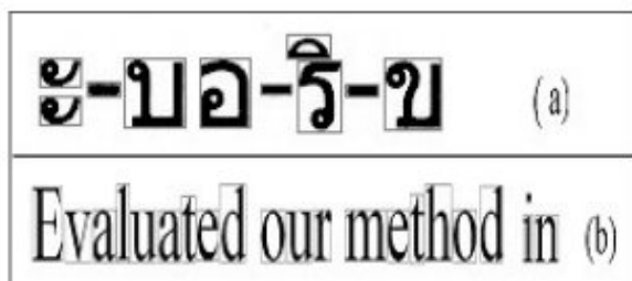
Fig.8. Bounding box of each component is shown in (a) Thai (b) English text.
