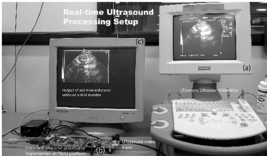
Fig. 5. The experimental real-time processing setup is shown in this figure. Input for the DM 642 based hardware (marked (b)) board is given from a Siemens Medical Ultrasound Machine (marked (a)) on the right of the figure and the processed output is being displayed on a separate RGB monitor (marked (c)) in real-time on the left of the figure. The board in front of the RGB monitor is the DM 642 based hardware.
