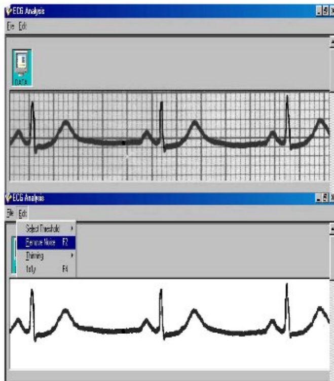
Fig. 3. (Upper) Original paper ECG record image and (lower) ECG signal after removal of background noise.
