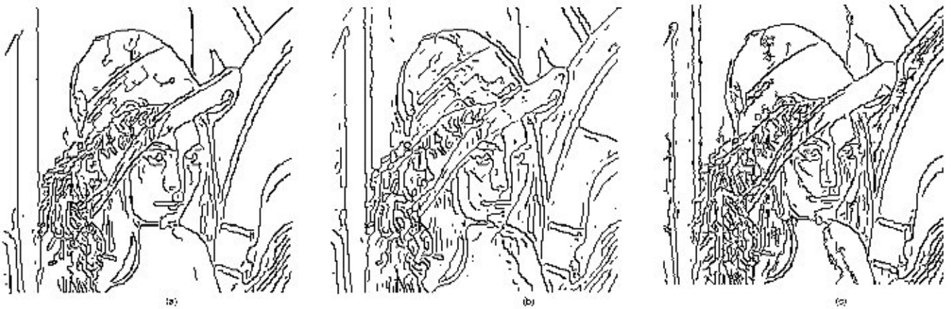
Fig. 6. Results on Lena image. (a) Proposed method ( h = 1.25, T_1 = 5, T_2 = 30 ). (b) Cumani's method ( \sigma = 1.5, T = 15 ). (c) Ruzon et al. 's method ( R = 1.5, low = 0.1, high = 0.3 ).
