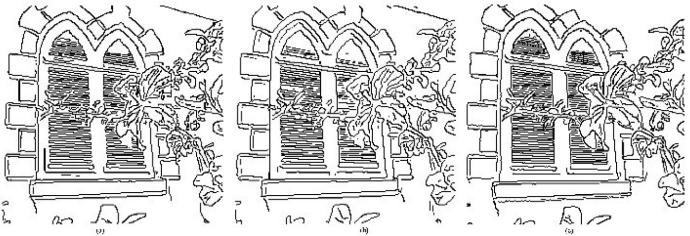
Fig. 7. Results on window image. (a) Proposed method ( h = 1.25, T_1 = 5, T_2 = 30 ). (b) Cumani's method ( \sigma = 1.5, T = 15 ). (c) Ruzon et al. 's method ( R = 1.5, low = 0.1, high = 0.3 ).
