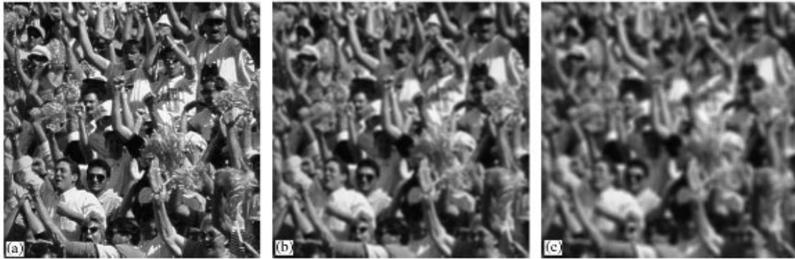
Fig. 2. Effect of mean filtering: (a) original crowd image; (b) Blurred image with n = 7 and (c) 11.
