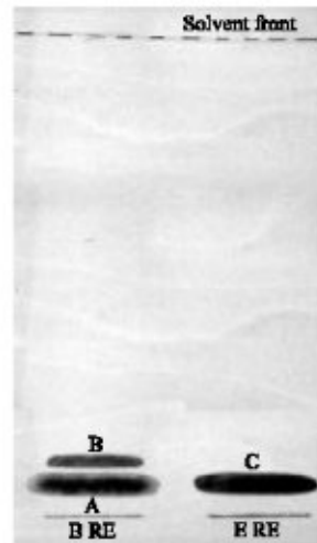
Fig. 3: Paper chromatographic run of root exudates of Bruguiera gymnorrhiza (B RE) and Excoecaria agallocha (E RE). The chromatogram shows two bands (A and B) in case of B RE and a single band (C) in case of E RE. Solvent system: n-butanol: acetic acid: water:4:1:1
