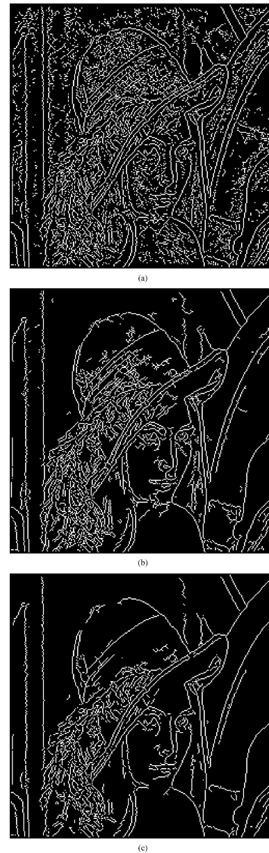
Fig. 12. Edges are detected from Lena image (Fig. 4) using Canny's method. Edge map (a) is obtained by taking \sigma = 1 , lower thresh = 0.03, and upper thresh = 0.04, which was used to get visibly good result for hand image [Fig. 8(b)]. Edge map (b) is obtained by taking \sigma = 0.75 , lower thresh = 0.0438, and upper thresh = 0.1094, which was used to get a visibly good result for dome image [Fig. 11(b)]. Edge map (c) is a very good result obtained for the parameter values \sigma = 1 , lower thresh = 0.0563, and upper thresh = 0.1406.
