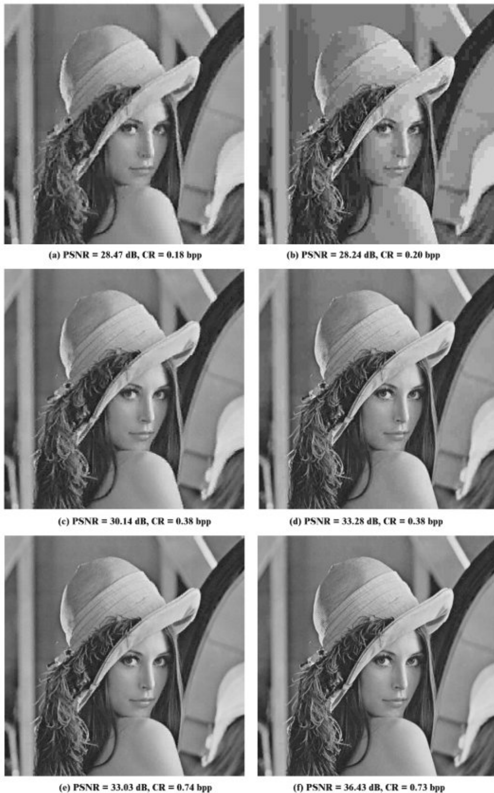
Fig. 6. (a), (c), (e) Compressed Lena images using proposed algorithm. (b), (d), (f) compressed Lena images using JPEG.
