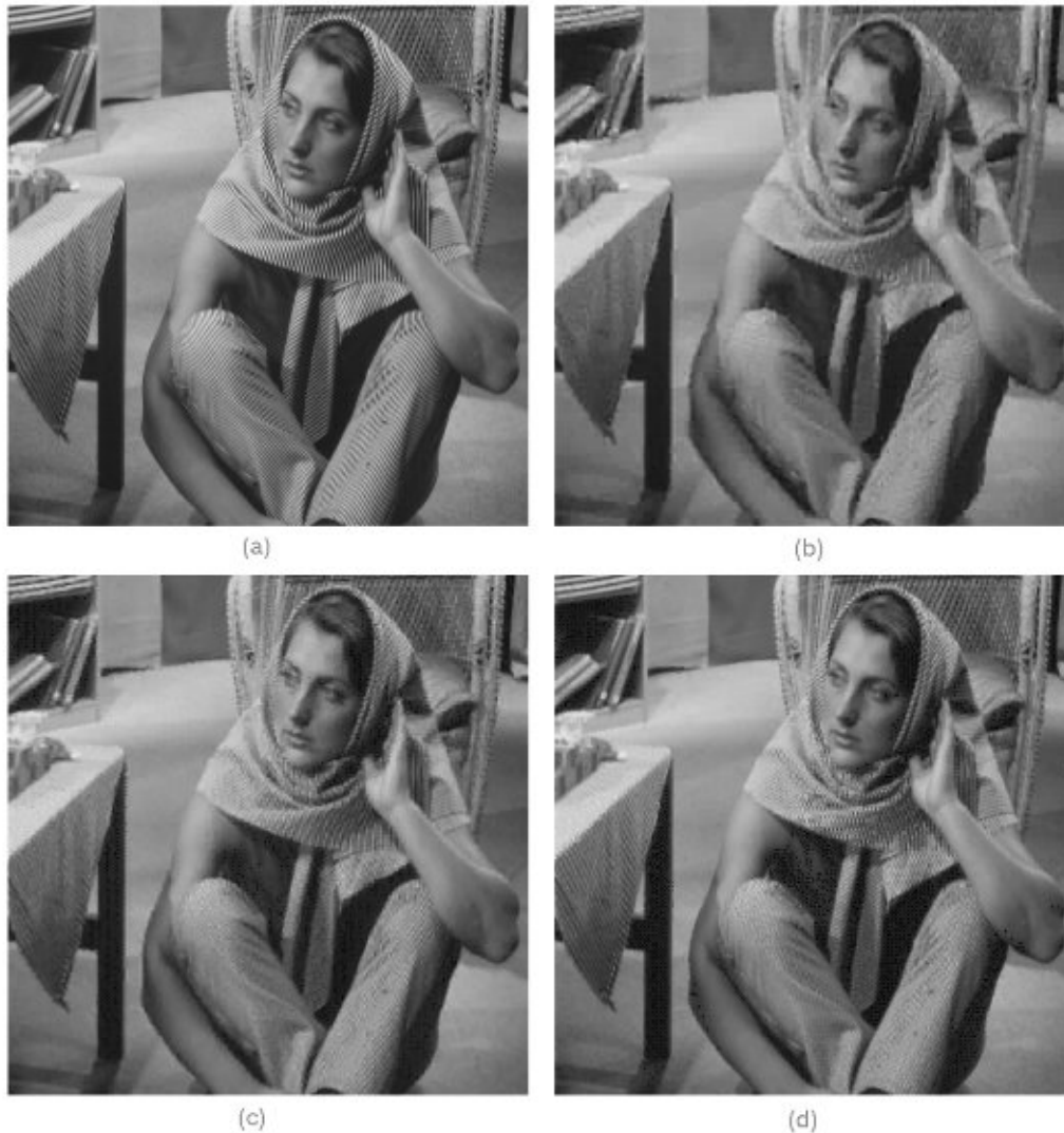
Fig. 7. Results on 512 \times 512 barbara image. (a) Original image. (b) Reconstructed image for VQ with 8 \times 8 blocks. (c) Reconstructed image for VQ with 4 \times 8 blocks. (d) Reconstructed image for VQ with 4 \times 4 blocks.
