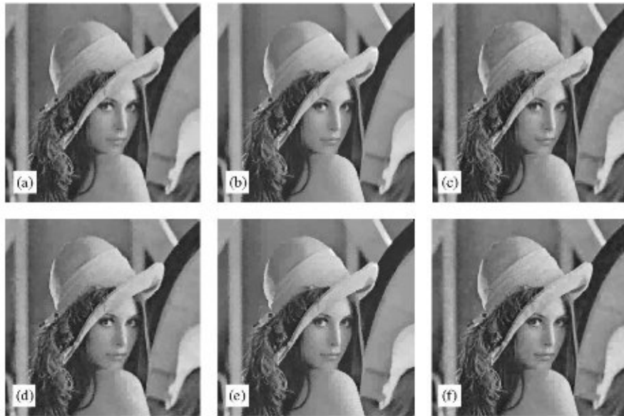
Fig. 8. Comparison of Lena image, (a) Algorithm 1 : \text{bpp} = 1.44 , \text{PSNR} = 30.577 , (b) Kamata : \text{bpp} = 1.45 , \text{PSNR} = 30.019 , (c) Algorithm 2 : \text{bpp} = 1.44 , \text{PSNR} = 31.222 , (d) Algorithm 1 : \text{bpp} = 1.28 , \text{PSNR} = 29.757 , (e) Kamata : \text{bpp} = 1.20 , \text{PSNR} = 29.163 , (f) Algorithm 2 : \text{bpp} = 1.34 , \text{PSNR} = 30.821 .
