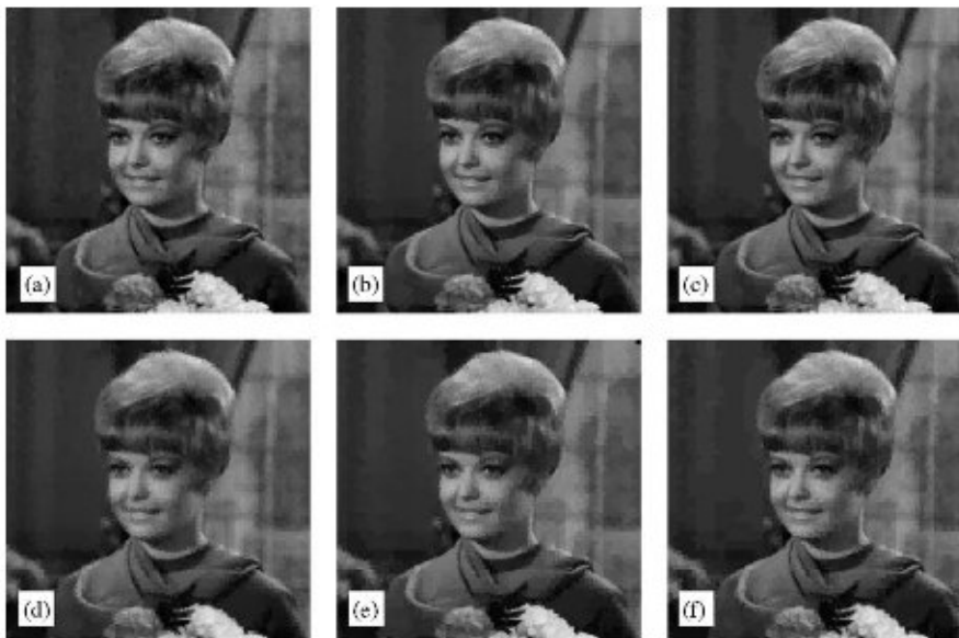
Fig. 9. Comparison of girl image, (a) Algorithm 1 : \text{bpp} = 1.09 , \text{PSNR} = 28.999 , (b) Kamata : \text{bpp} = 1.01 , \text{PSNR} = 30.361 , (c) Algorithm 2 : \text{bpp} = 1.07 , \text{PSNR} = 30.436 , (d) Algorithm 1 : \text{bpp} = 0.60 , \text{PSNR} = 27.346 , (e) Kamata : \text{bpp} = 0.68 , \text{PSNR} = 28.442 , (f) Algorithm 2 : \text{bpp} = 0.68 , \text{PSNR} = 28.811 .
