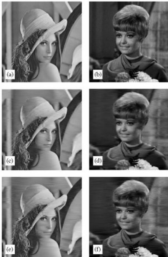
Fig. 5. Results for Algorithm 1 ((c), (d)) and Algorithm 2 ((e), (f)) due to raster scan, (a) input Lena image, (b) input girl image, (c) bpp = 1.47, PSNR = 30.574, (d) bpp = 1.40, PSNR = 28.075, (e) bpp = 1.71, PSNR = 30.020, (f) bpp = 1.539, PSNR = 30.169.
