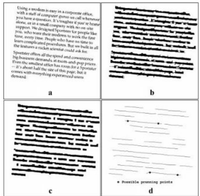
Fig. 2a. Original document in binary b closing original binary image with 4 \times 12 SE c opening the closed image with 5 \times 5 SE d after transition and rejection of small lines operation
