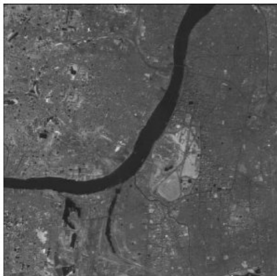
Fig. 10. SPOT image of Calcutta in the near infra red band (the image is enhanced by a factor of 75%).
