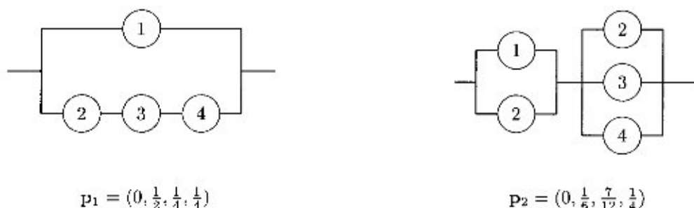
Figure 5. Systems for which \mathbf{p}_1 \leq^s \mathbf{p}_2 , \mathbf{p}_1 \not\leq^{hr} \mathbf{p}_2 , \mathbf{p}_1 \not\leq^{lr} \mathbf{p}_2 .
