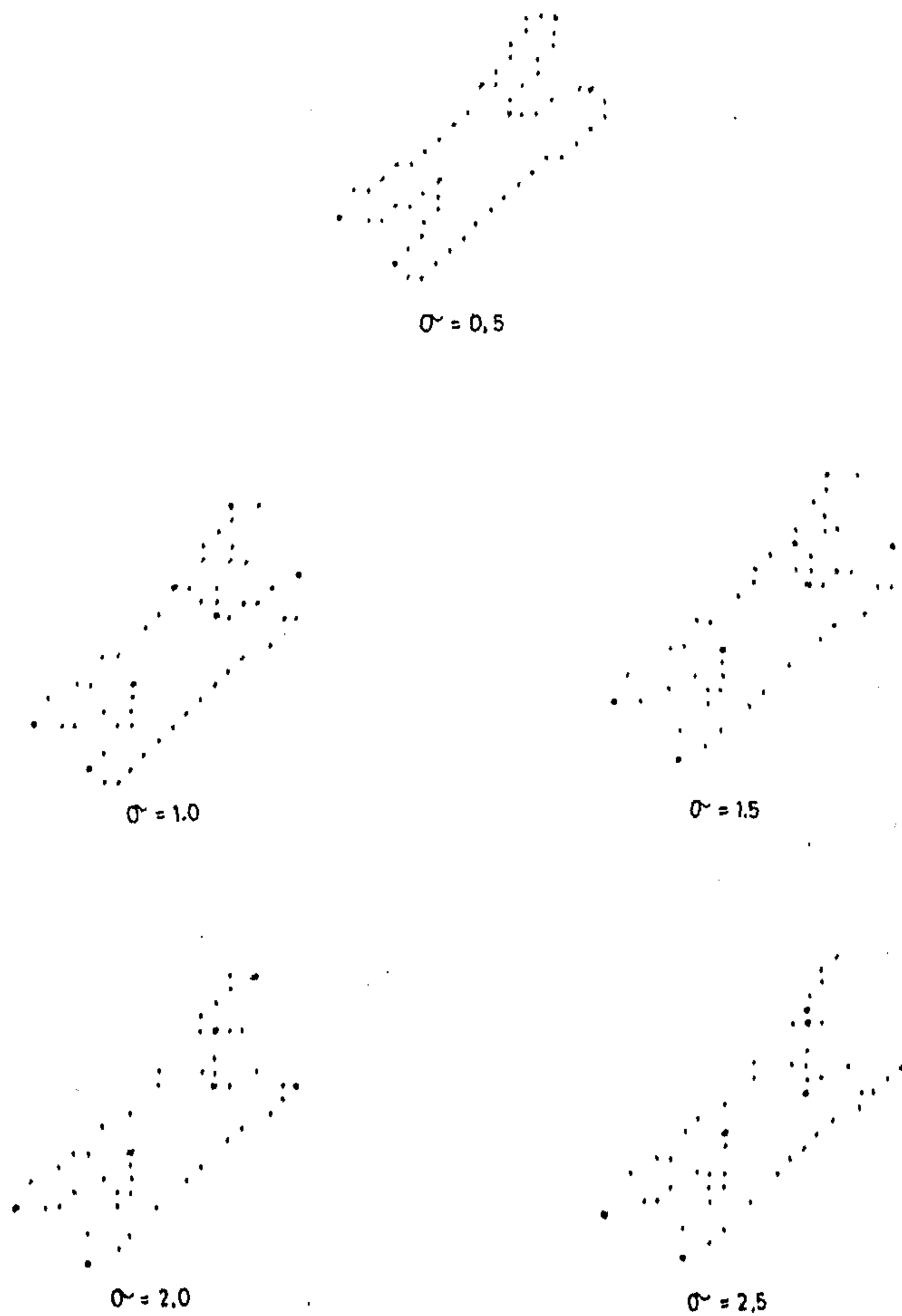
Figure 11.12: The noisy chromosome at varying noise levels. The corners are indicated by bold solid circles.
