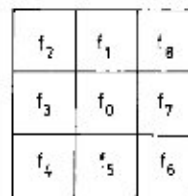
Fig. 2. A 3 \times 3 window centered at candidate pixel (j, k) having gray level f_0 .
