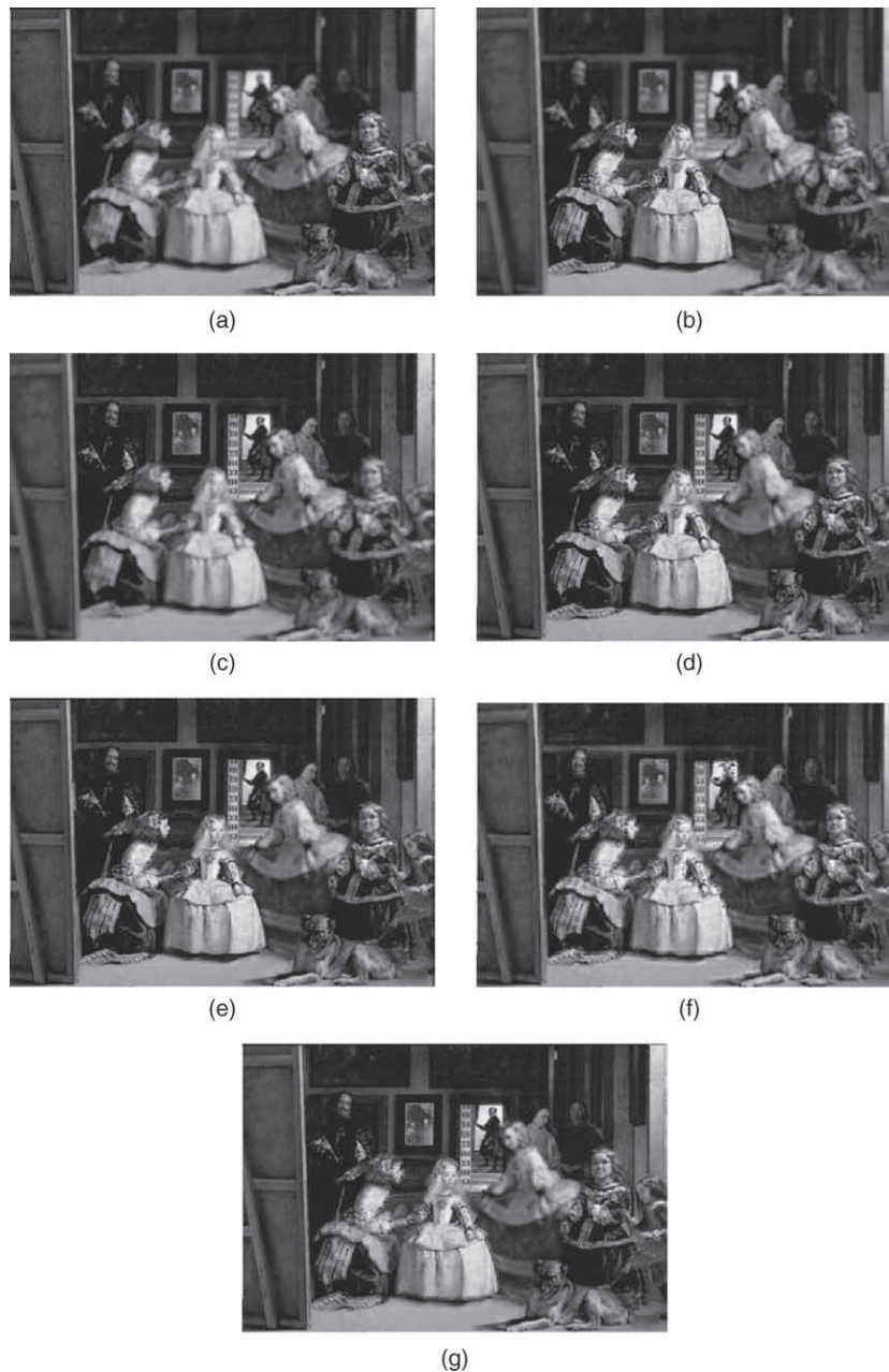
Fig. 5. Original multifocus images and the fused images by various algorithms. (a) Near focused image, (b) middle focused image, (c) far focused image, (d) fused image with proposed algorithm, (e) fused image with gradient method with majority filtering, (f) fused image with Haar wavelet method, (g) fused image with weighted averaging.
