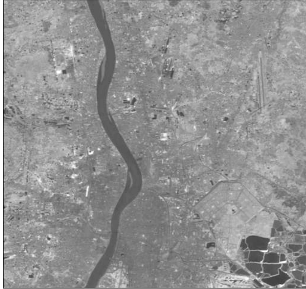
Figure 3. IRS Image of Kolkata in the Near Infra Red Band with Histogram Equalization
