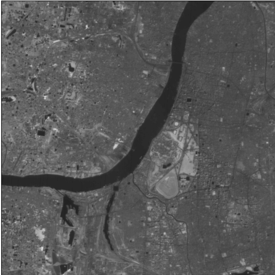
Fig. 6. SPOT image of Calcutta in the near infra red band (Band 3). The image is histogram stretched.
