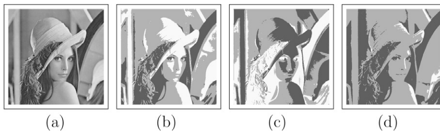
Fig. 10. (a) Original image of Lena. Segmented image by: (b) APC-best S.Dbw and APC-best DB , (c) k -means, and (d) mean shift.
