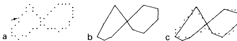
Figure 3. (a) A figure-8 curve. (b) Polygonal approximation of (a). (c) Overlap of (b) on (a).
