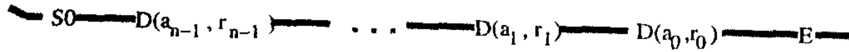
Figure 6.8: ssDNA representation of the n -bit number A = (a_{n-1} \dots a_1 a_0)
