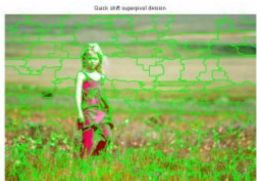
Figure 4.2: After superpixel division. Superpixel has been created in LAB space using quick shift. Green lines represent the boundary of individual superpixels.
