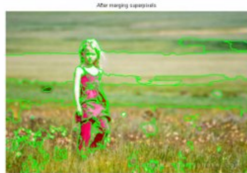
Figure 4.3: After merging superpixels using mean of R,G and B value of each individual superpixel.
