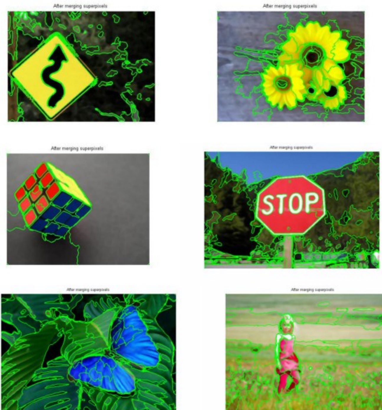
Figure 5.9: Merging the smaller superpixels based on the differences between the average of R, G and B values between them.
