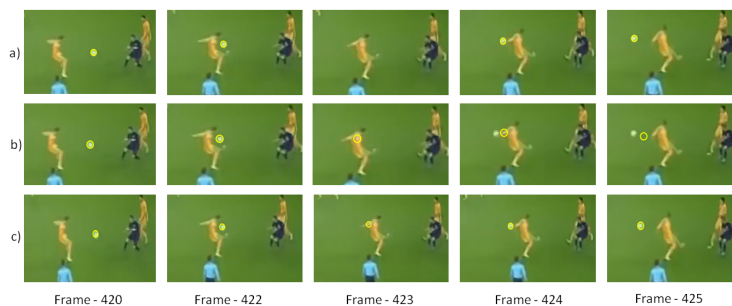
Figure 3.6: Performance evaluation when short time full occlusion occurs, (a) Ground truth result, (b) Result of mean shift algorithm based on color histogram matching, (c) Result of our football tracking algorithm
