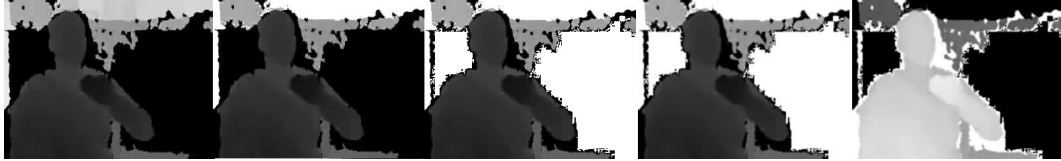
FIGURE 3.2: From left to right: (a) Original frame from video (b) After background removal (c) After using connected components to filter noise (d) After applying gaussian filter (e) Final inverted image
