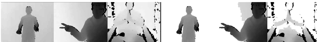
FIGURE 3.1: The first three images on the left are the original extracted depth frames. The latter three images have the background removed from them.
