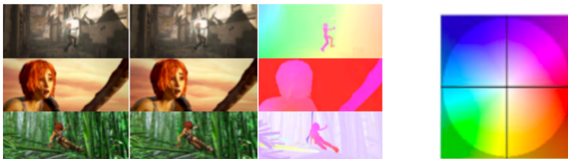
Figure 3.1: (Left) Example from MPI-Sintel Dataset: image1, image2, ground truth flow prediction. (Right) Coding Color of the flow vectors.
