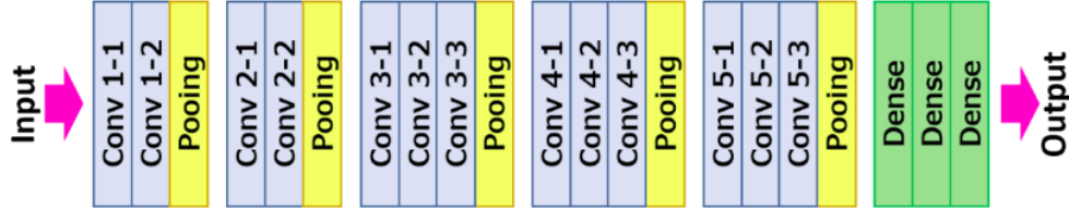
Figure 1.2: Diagram of VGG16 architecture [4]
