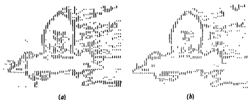
Figure 10. (a) Thresholded version of Fig. 8(c) using normal histogram thresholding techniques when thresholded at edge intensity level 4; (b) thresholded version of Fig. 8(c) using the same technique with level of threshold 6.
