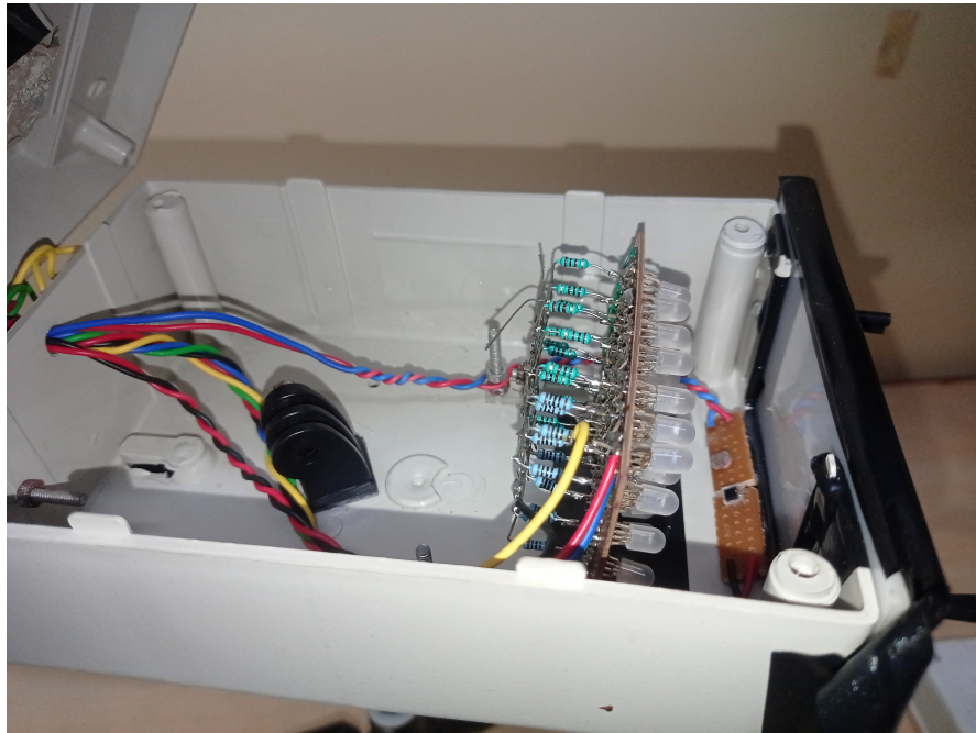
FIGURE 7.1: The Light Emitting diodes soldered together in the device
