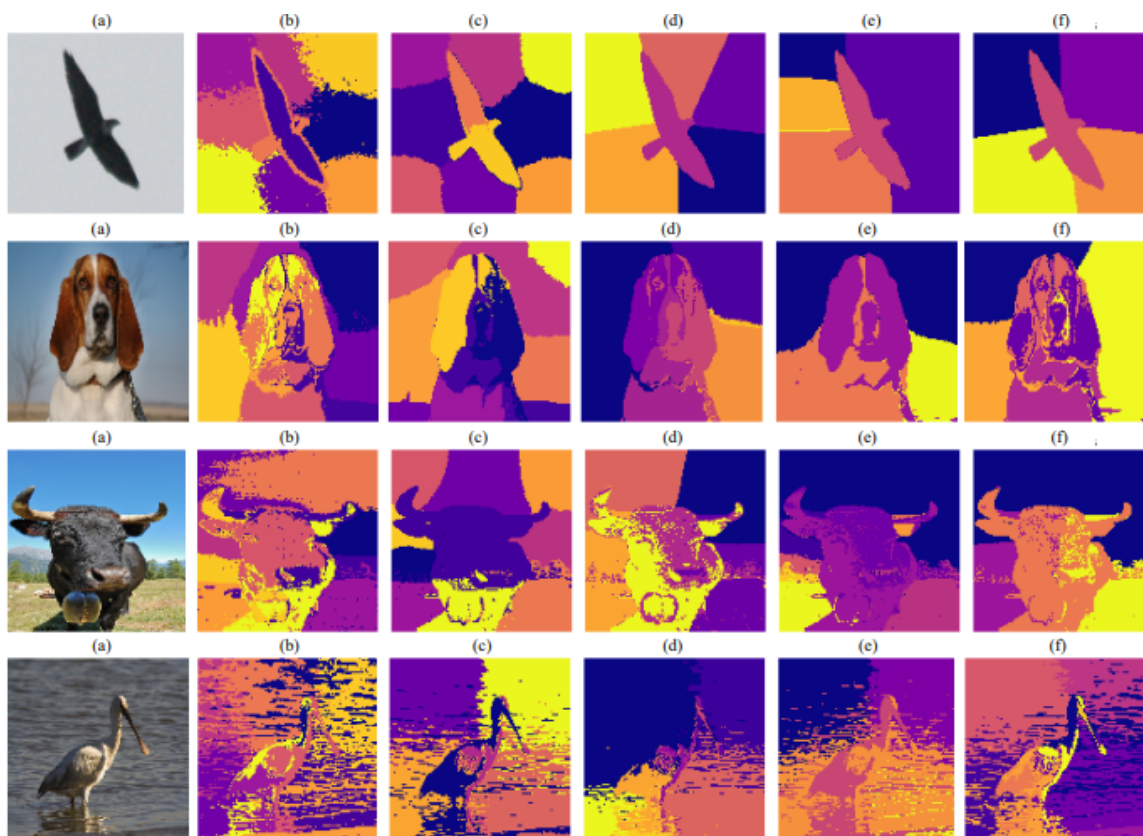
Figure 6.2: Qualitative segmentation results on PASCAL VOC 2012 [13]. Columns show: (a) Input image, (b) GMS, (c) GridShift, (d) QuickMeanShift, (e) GBMS, (f) HypeGBMS (ours). HypeGBMS consistently preserves object boundaries and avoids over-segmentation.
