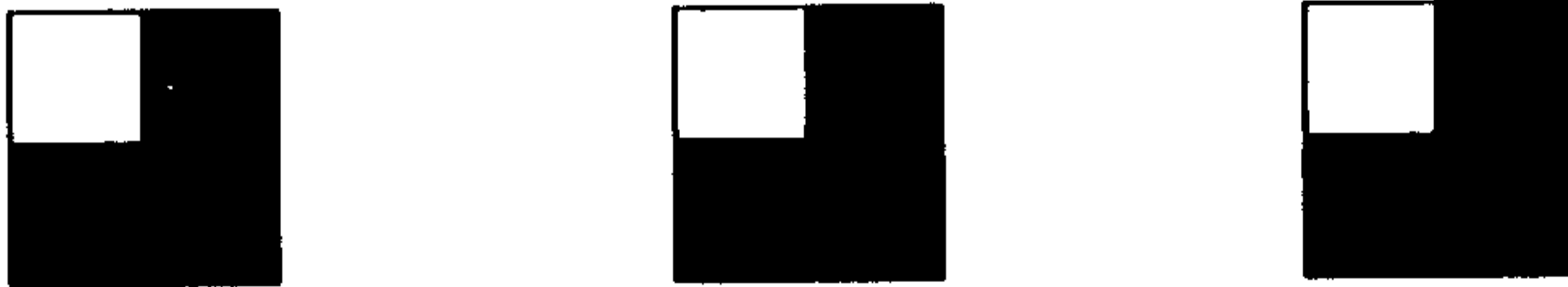
Fig :5 A square image can always be oriented so that the brightness, or average values, of its quadrants fall into one of these canonical positions.
