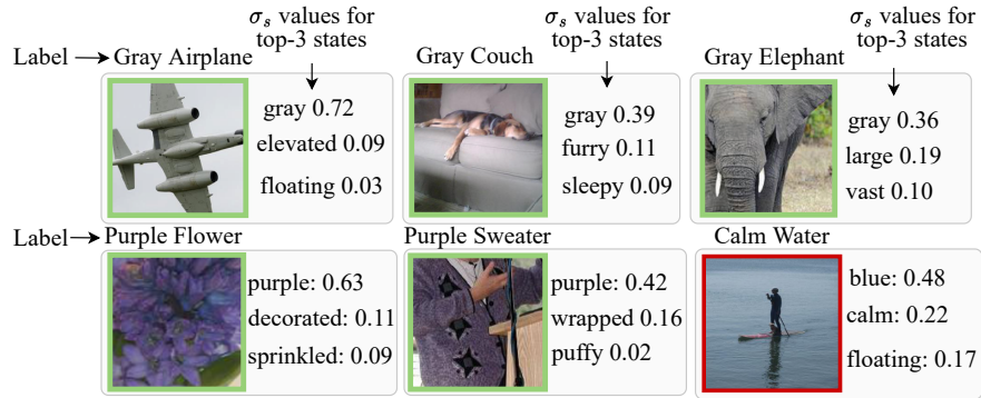
Figure 4.8: Results from the test set of C-GQA dataset and the corresponding top-3 \sigma_s^i values as predicted by SWPG module. For an input test image, if the highest value of \sigma_s^i , ( i \in \{1, 2, \dots, N_s\} ) is obtained for the ground truth state, then the image is shown in green border else in red border.
