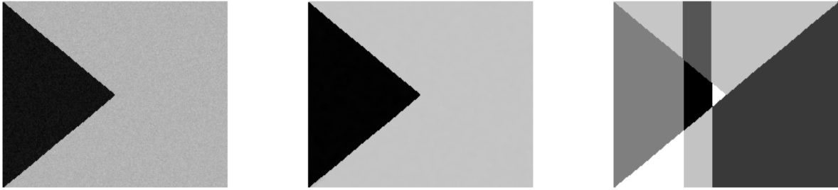
Figure 3.2: Demonstration of partitioning of the pixels in the test image. Images from left to right are the noisy image, the denoised image by the proposed method, and the estimated partitions, respectively. The partitions are represented by different shades. Note that the estimated partitions are subsets of the true partitions.
