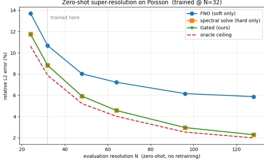
Figure 6.11: Zero-shot super-resolution on the Poisson equation. The FNO and the gate are trained at N = 32 (gate also at N \in \{24, 48\} ) and evaluated untouched at every grid, including N \in \{64, 96, 128\} unseen during training. The soft FNO error stays controlled and decreases under upsampling — the super-resolution result — while the gated model (green) sits on or below both pure paths at every resolution and tracks the per-mode oracle ceiling.
