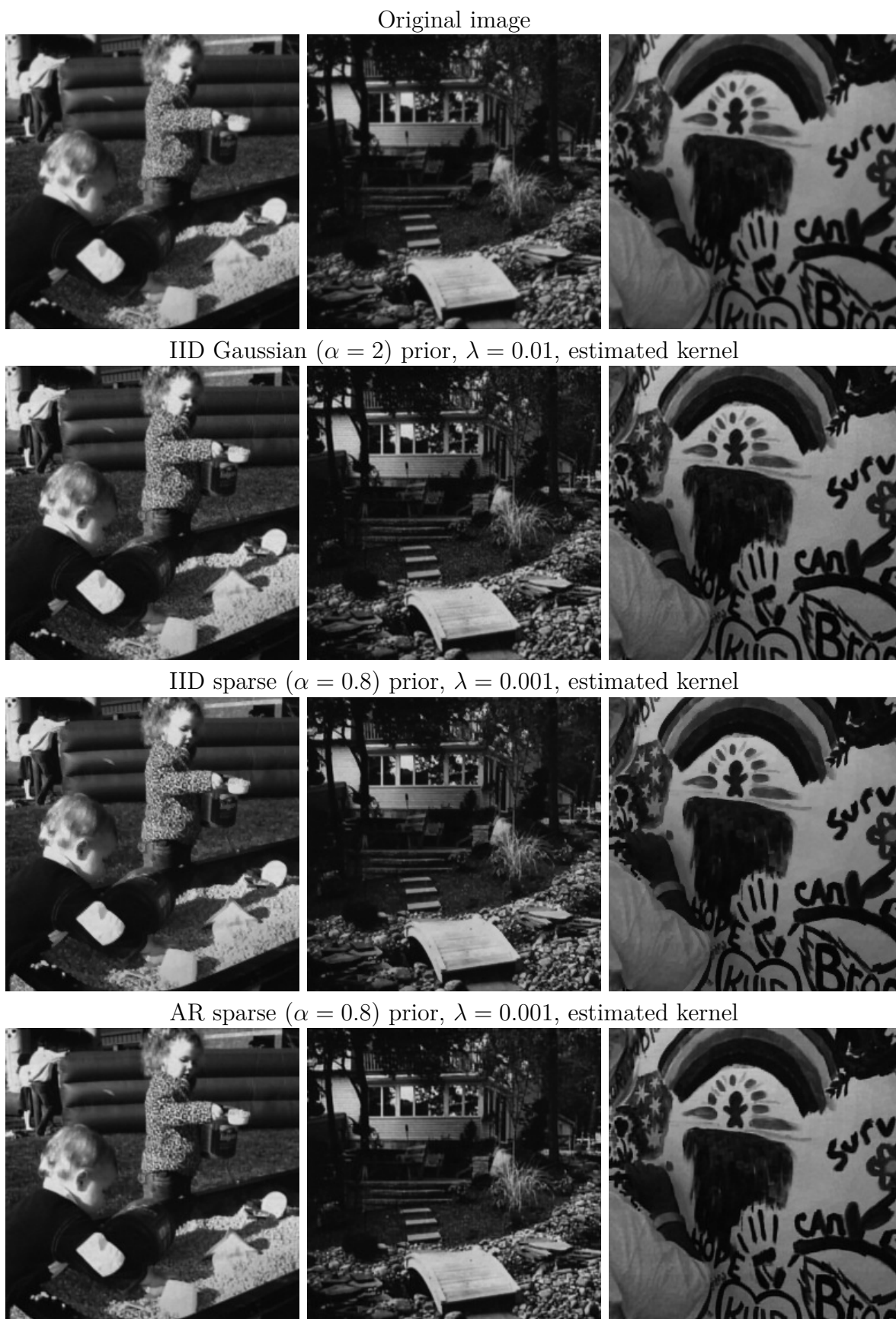
Figure 6.4: Deconvolution of the first three test images using the blur kernels estimated from the input images, shown in Figure 5.7.
