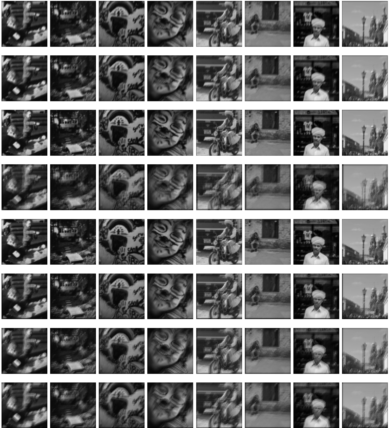
Figure 1.6: Synthetically blurred images for all combinations of the eight test images (columns) and eight test kernels (rows). There is no additional noise, except for the integer rounding inherent in storing 8-bit images.
