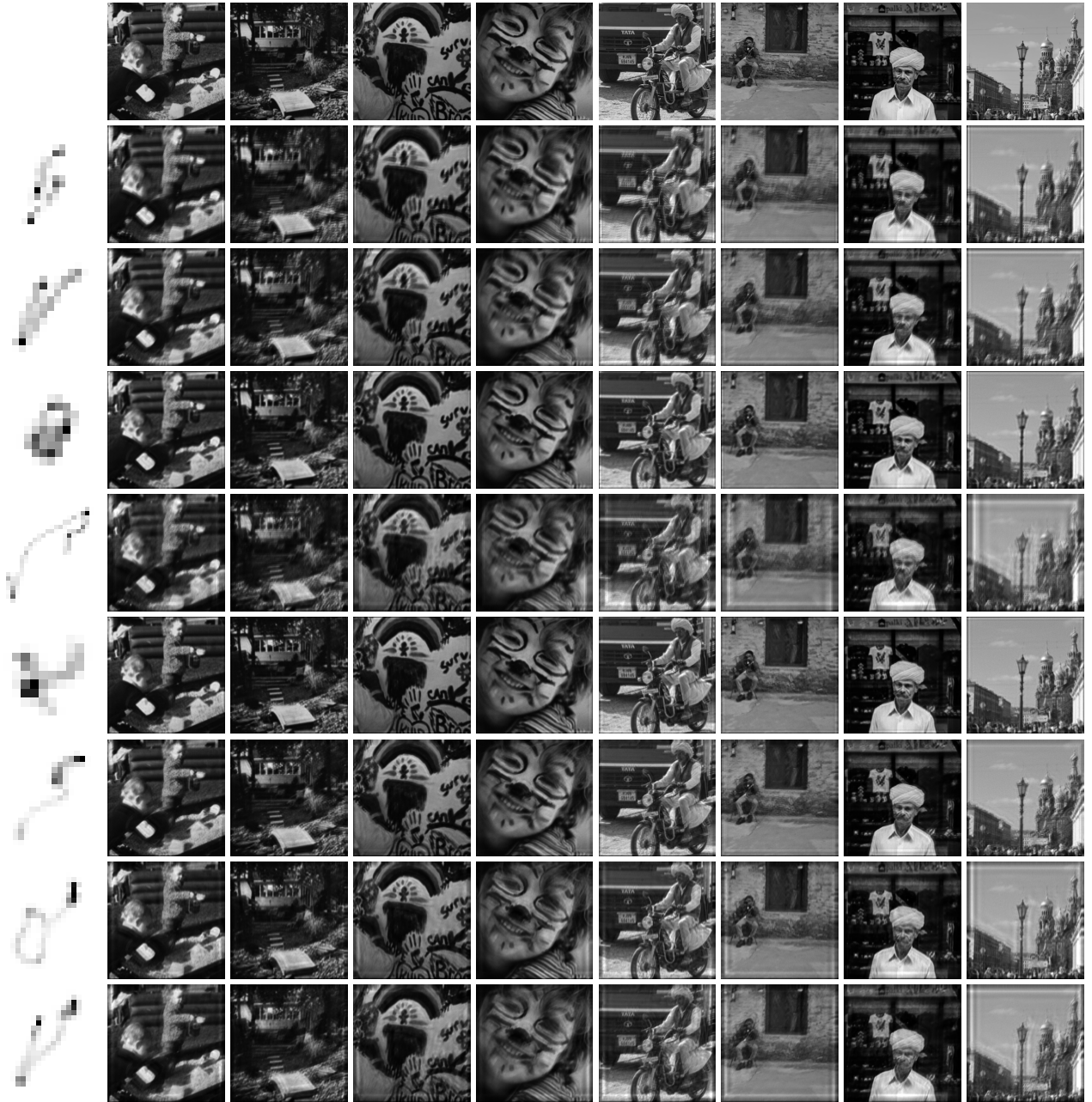
Figure 2.4: Results of non-blind deconvolution using the Richardson-Lucy algorithm for all image-kernel combinations shown in Figure 1.6 with additional noise ( S = 100 ).
