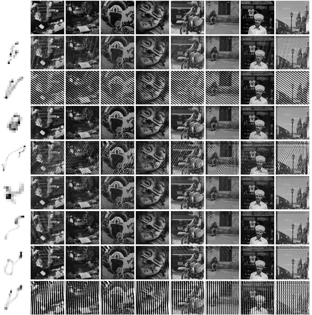
Figure 2.2: Results of non-blind deconvolution using the direct inversion method for all image-kernel combinations shown in Figure 1.7 with additional noise ( S = 100 ).
