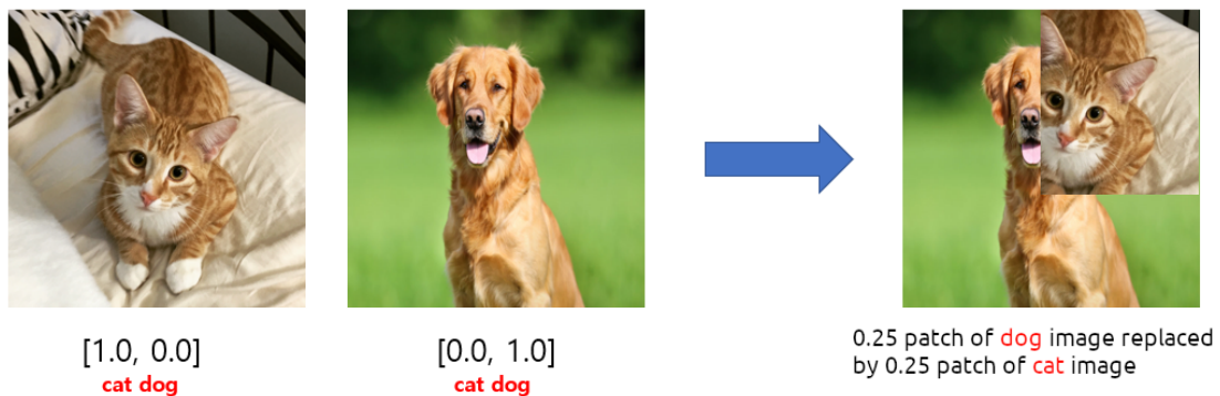
Figure 2.4: Cutmix demonstrated between two images of different classes in cat dog dataset
