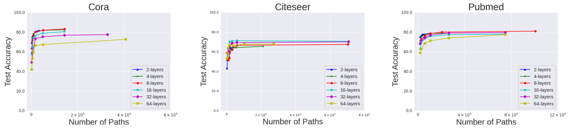
Figure 2.5: Test accuracy of RPE-GNN is observed by varying the number of random paths for different depths of the architecture. Test accuracy increases when the number of sampled paths is increased. The model with more depth needs more random paths to produce optimal results.
